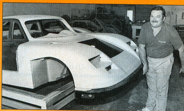
Can you believe the unitized frame-and-body weighs only 275 pounds?
